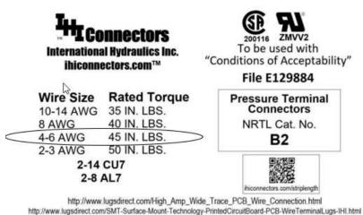
7. Both 6.0 AWG and 5.2 AWG fall into the 45 in-lb (5.1 N-m) torque rating of AWG range 4-6. UL486F and UL486AB allow the B/C torque to be used as though the Flex strands were converted to rigid strands or for 10-4 AWG flex stranded as though converted to solid wire. See Ferrule Conversion Chart here.
